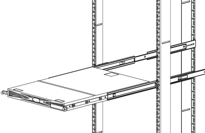
A technical line drawing showing a server being inserted into a rack enclosure. The server is shown from a perspective view, with its front bezel facing left and its rear panel facing right. The server is being pushed into the rack enclosure, which has the outer slide members installed. The server's internal slides are aligning with the rack's rails. The server is shown partially inserted, with its front bezel still outside the enclosure. |
