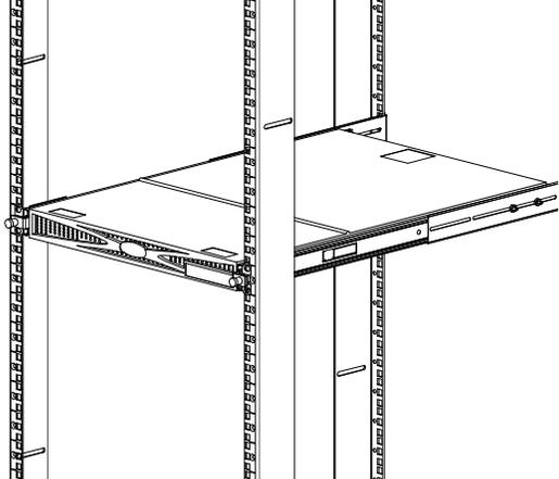
A technical line drawing showing the server fully inserted into the rack enclosure. The server's front bezel is now flush with the rack's front panel. Two thumbscrews are shown on either side of the bezel, being tightened to secure the server in place. The server's front panel is now fully visible, and the rack enclosure is closed.                                                                                                             |
