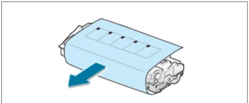
4. Shake the cartridge from side to side 5 or 6 times to distribute the toner evenly inside the cartridge.
