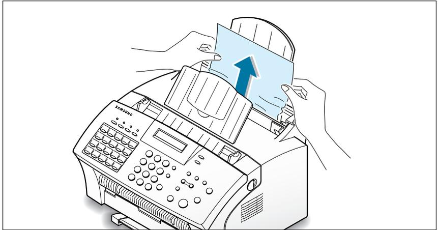
2. After you have removed the jammed paper, load the paper with the print side facing you.
