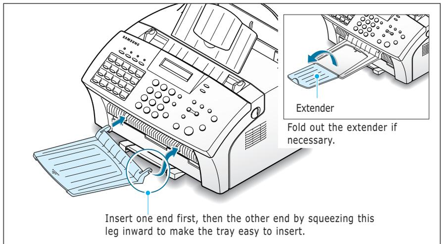
**Note:** The SF-530 series is shipped with the paper output tray already installed. Extend the tray to use.
