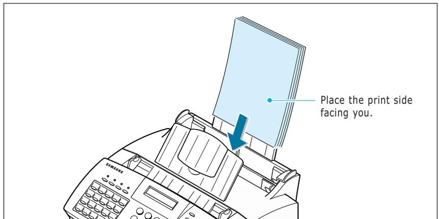
4. Adjust the paper guides to the width of the print media. Slide the guides until they lightly touch the stack of print media. Do not bend the print material.
