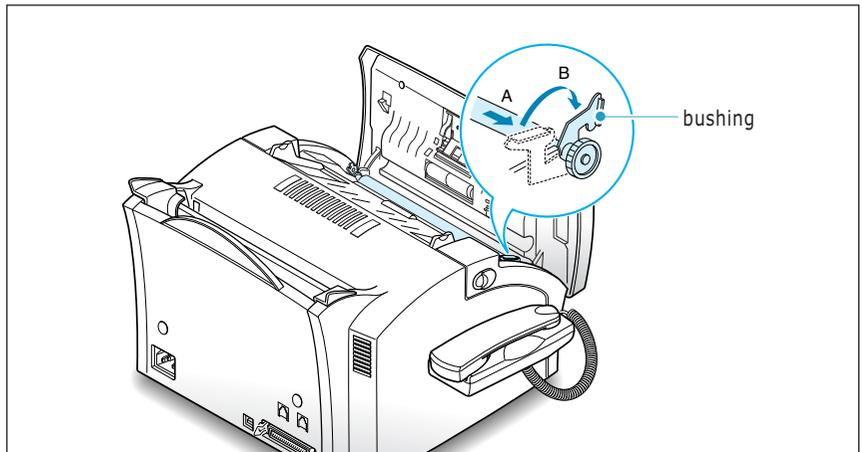
3. Wipe the roller surface with a soft cloth dampened with water.
