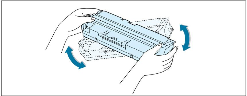
5. Find the cartridge slots inside the machine, one on each side. Grasp the handle and slide the cartridge down between the cartridge slots until it drops into place.
