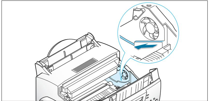
5. Grasp the handle at the front of the cartridge and slide it down between the cartridge slots, and push it firmly.
