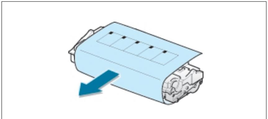
3. Shake the cartridge from side to side 5 or 6 times to redistribute the toner evenly inside the cartridge.
