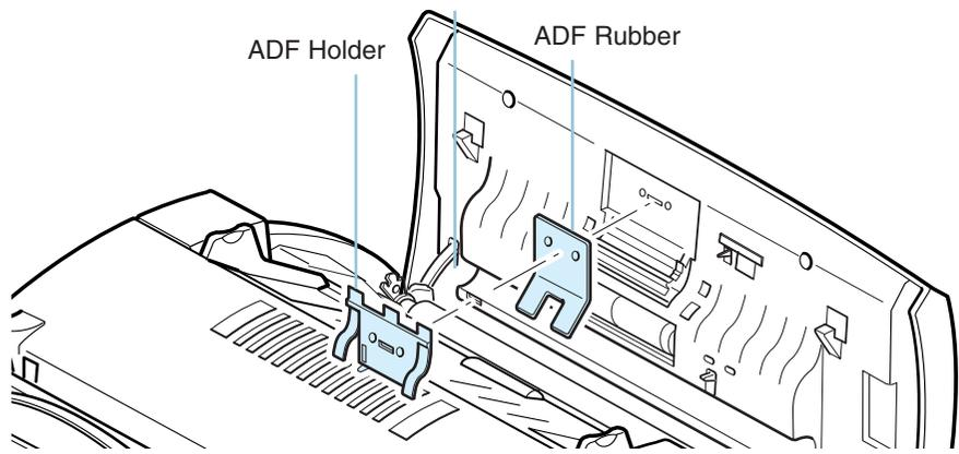
3. Apply upward pressure to release the two locking tabs on each side of the assembly.
