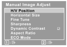
**H./V. Position (Horizontal/Vertical Position)** moves the screen image left or right and up or down.
