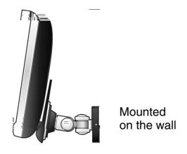
**5** Attach the ViewPanel to the wall, following the instructions in the wall-mounting kit.
