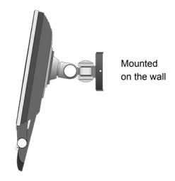
**5.** Attach the LCD display to the wall, following the instructions in the wall-mounting kit.
