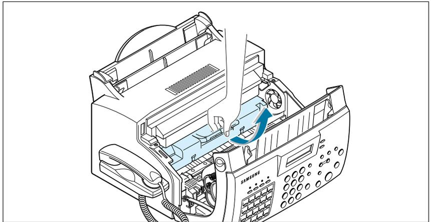
3. Unpack a new toner cartridge from its plastic bag, and then remove the paper rolled the cartridge.
