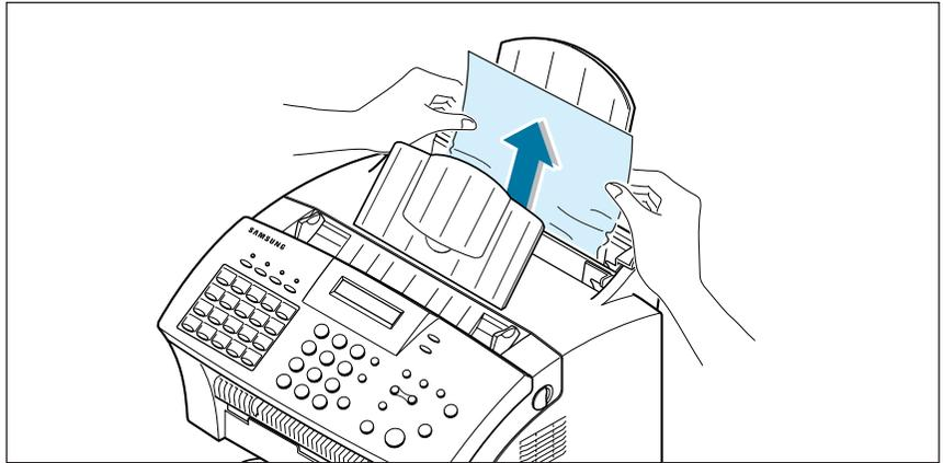
2. After you have removed the jammed paper, load the paper with the print side facing you.
