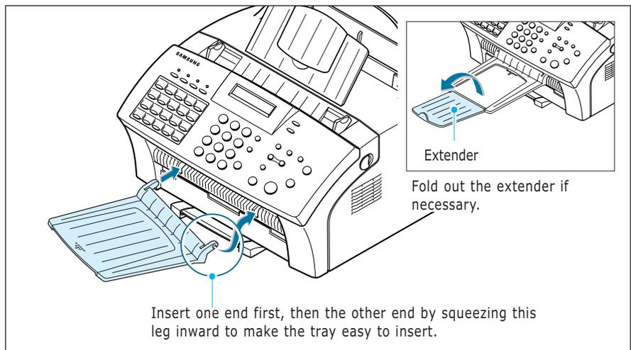
**Note:** The SF-555P is shipped with the paper output tray already installed. Extend the tray to use.
