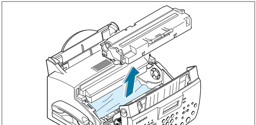
3. Remove the jammed paper by carefully pulling it out of the machine.
