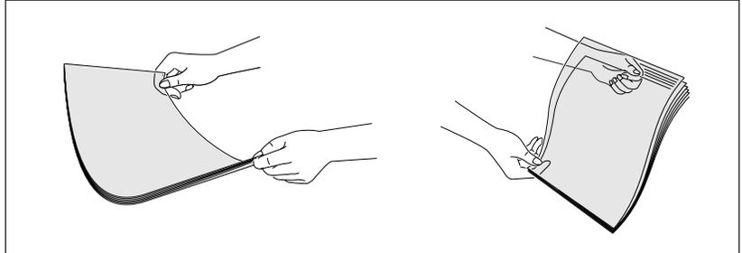
3. Load the print material into the paper tray. Load only as much paper as will fit beneath the lip protruding from the paper-length adjuster. Neatly stacking the paper before loading will help prevent print problems. Do not mix types. See the following directions to load each type of print material.
