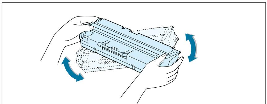
3. Reinstall the cartridge and close the cover.
