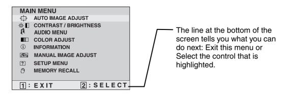
**NOTE:** All OnView menus and adjustment screens disappear automatically after about 30 seconds. This time period is adjustable through the Setup menu and the OSD timeout control described on page 10.
