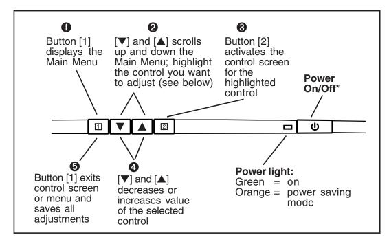
\* The monitor <u>automatically</u> degausses each time you turn it on, removing the buildup of magnetic fields that can affect color purity and convergence. To prevent possible damage, if you turn the monitor off, then immediately on again, wait 20 minutes before doing this again. Do not turn the monitor on and off repeatedly. To manually degauss the monitor, see the instructions on page 9.
