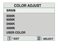
**sRGB** — sRGB is quickly becoming the industry standard for color management, with support being included in many of the latest applications. Enabling this setting allows the LCD display to more accurately display colors the way they were originally intended. Enabling the sRGB setting will cause the Contrast and Brightness adjustments to be disabled.
