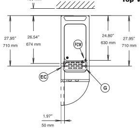
EC Electrical connection Gas connection Filtered Cold Water Inlet
