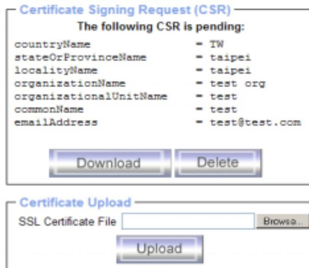
**Figure 6-24. SSL Certificate Upload**
