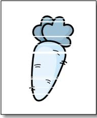
Cleaning your print cartridges can improve the quality of printing. If your printed page is missing lines or dots or contains ink streaks, clean the print cartridges as described in this section.
