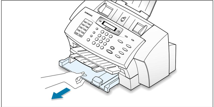
2. Slide the paper-width and paper-length adjusters out as far as possible to make room for the paper.
