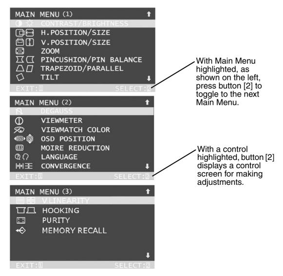
To select a control you want to adjust, press the arrow buttons on the front control panel of your monitor (▼▲) and scroll through the choices.
