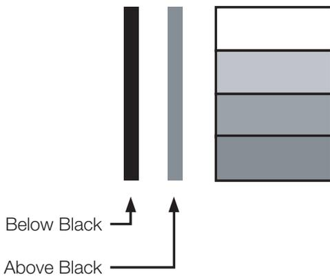
**Figure 4-2. Typical PLUGE Pattern for Adjusting Brightness**
