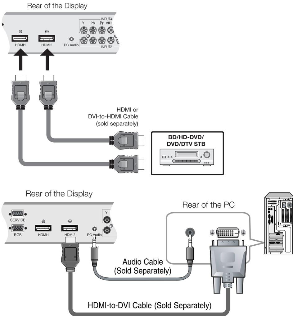
**Figure 3-2. HDMI Connections**
