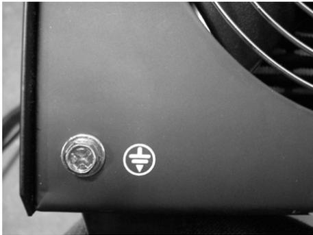
1. Attach a ground wire of at least 14 Ga. thickness (not supplied) to the screw on the lower left of the back of the tool case.
