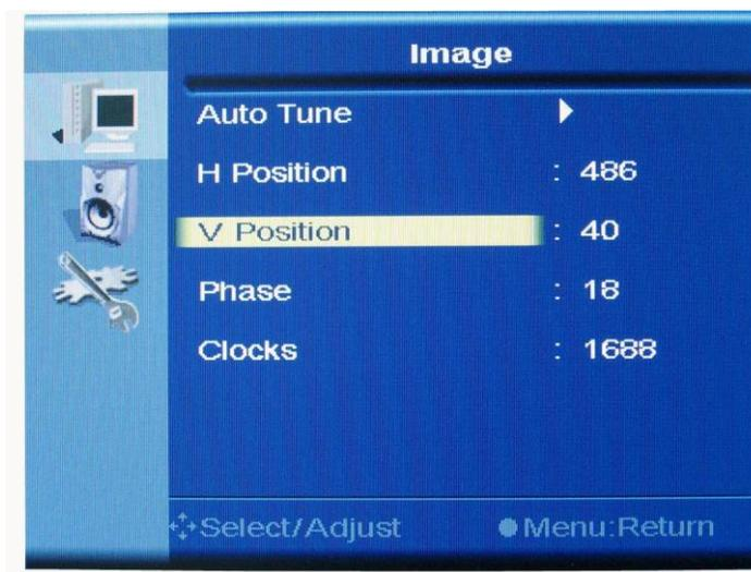
b. Press UP or DOWN to move the vertical position of OSD . Then press “1” to confirm the adjustment and back to Image menu.
