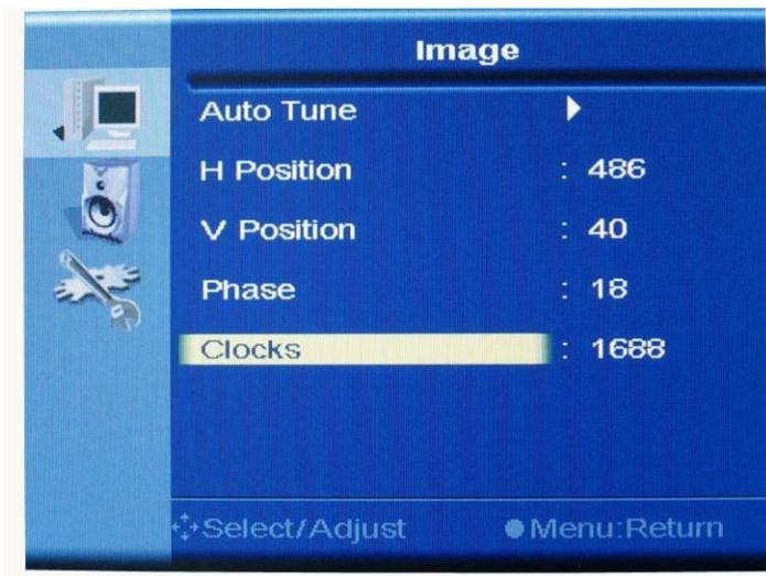
b. Press UP or DOWN to adjust the clock of signal. Then press “1” to confirm the adjustment and back to Image menu.
