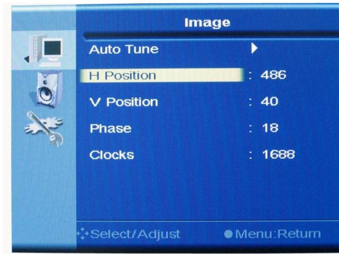
b. Press UP or DOWN to adjust the horizontal position. Then press “1” to confirm the adjustment and back to Image menu.
