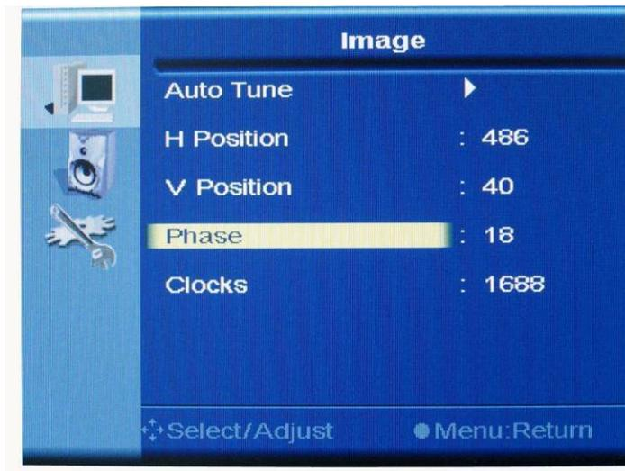
b. Press UP or DOWN to adjust the phase of signal. Then press “1” to confirm the adjustment and back to Image menu.
