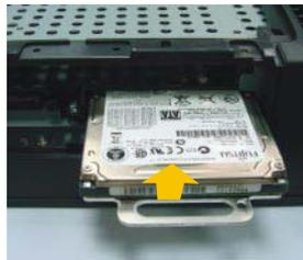
3. Secure the Hard Drive to the touchcomputer using the screw.
