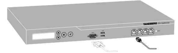
Connect the Ethernet LAN cable to socket LAN 1. Connect the null modem cable between the Data socket and a PC.
