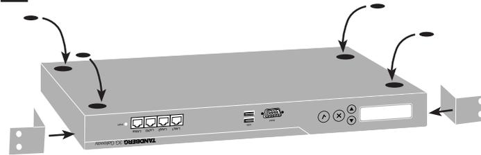
Mount the rack ears and/or rubber feet, if applicable, and turn the unit back on its feet or mount it in the rack.
