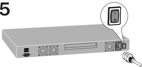
Connect the power cable and turn on the 3G Gateway. Use the LCD display of the unit to set the IP address – see *Configuring the 3G Gateway* in the User Manual for details, or...
