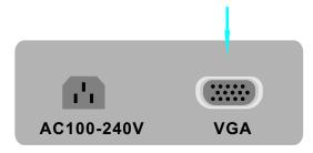
3. Plug the power connector into the AC In port port at the rear of the monitor.
