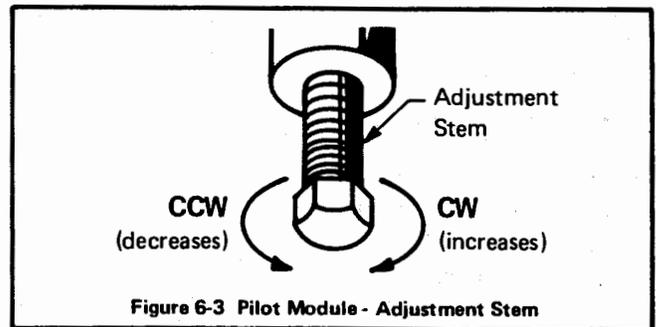
Figure 6-3 Pilot Module - Adjustment Stem
