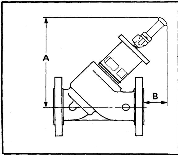
Figure 4-3, Table 4-3 - Clearance Dimensions - Cylinder Removal
