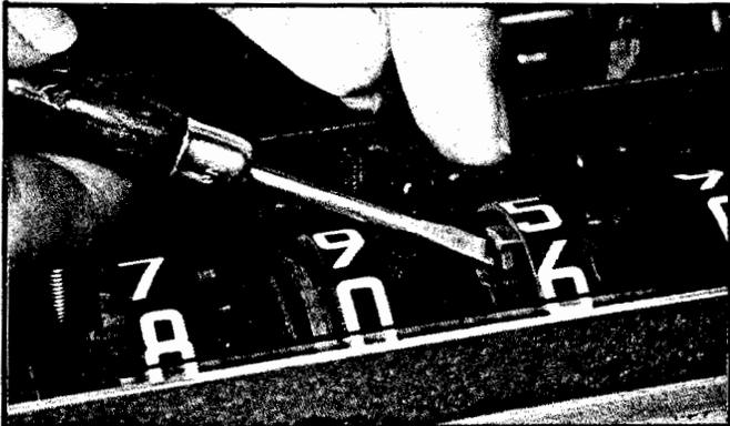
Figure 6-8 Removing Insert from Notch on Second Wheel.
