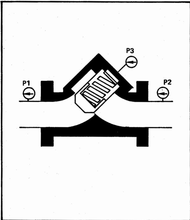
**Closed Position:** The valve is closed because (P1 is less than the spring force in the seated position or; (P2) is greater than (P1).
