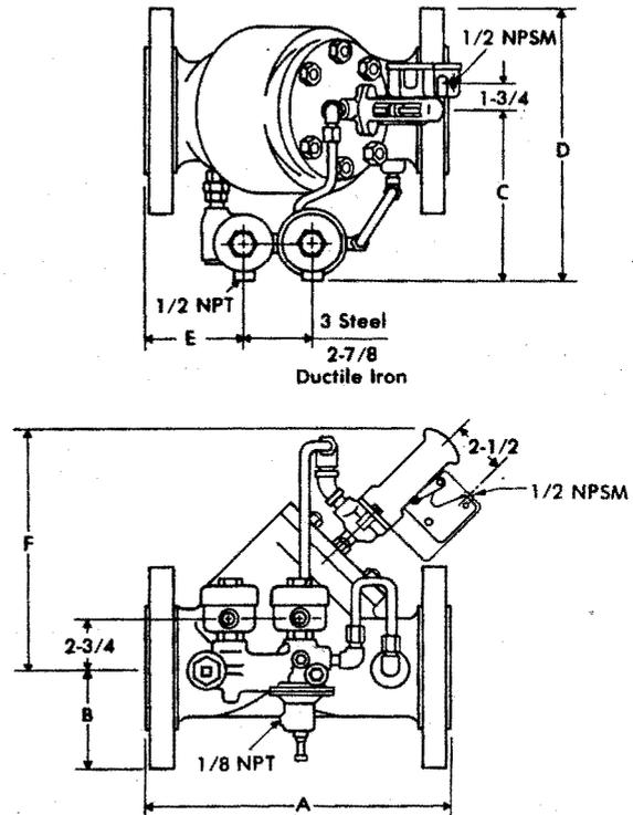
Figure 4-1 Physical Dimensions (In-Line).
