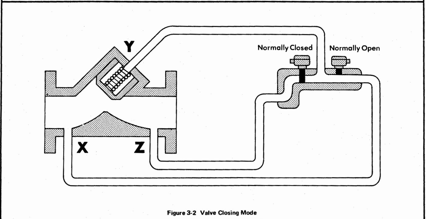
Figure 3-2 Valve Closing Mode
