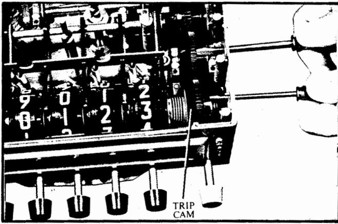
Figure 6-6 Trimming the Right-Hand Wheel.
