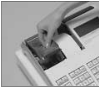
Step 2 Open the platen arm.
