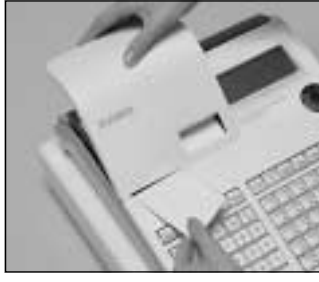
Step 3 Ensuring the paper is being fed from the bottom of the roll, lower the roll into the space behind the printer.
