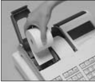
Step 3 Ensuring the paper is being fed from the bottom of the roll, lower the roll into the space behind the printer.
