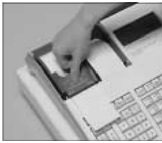
Step 5 Close the platen arm slowly until it locks steadily.
