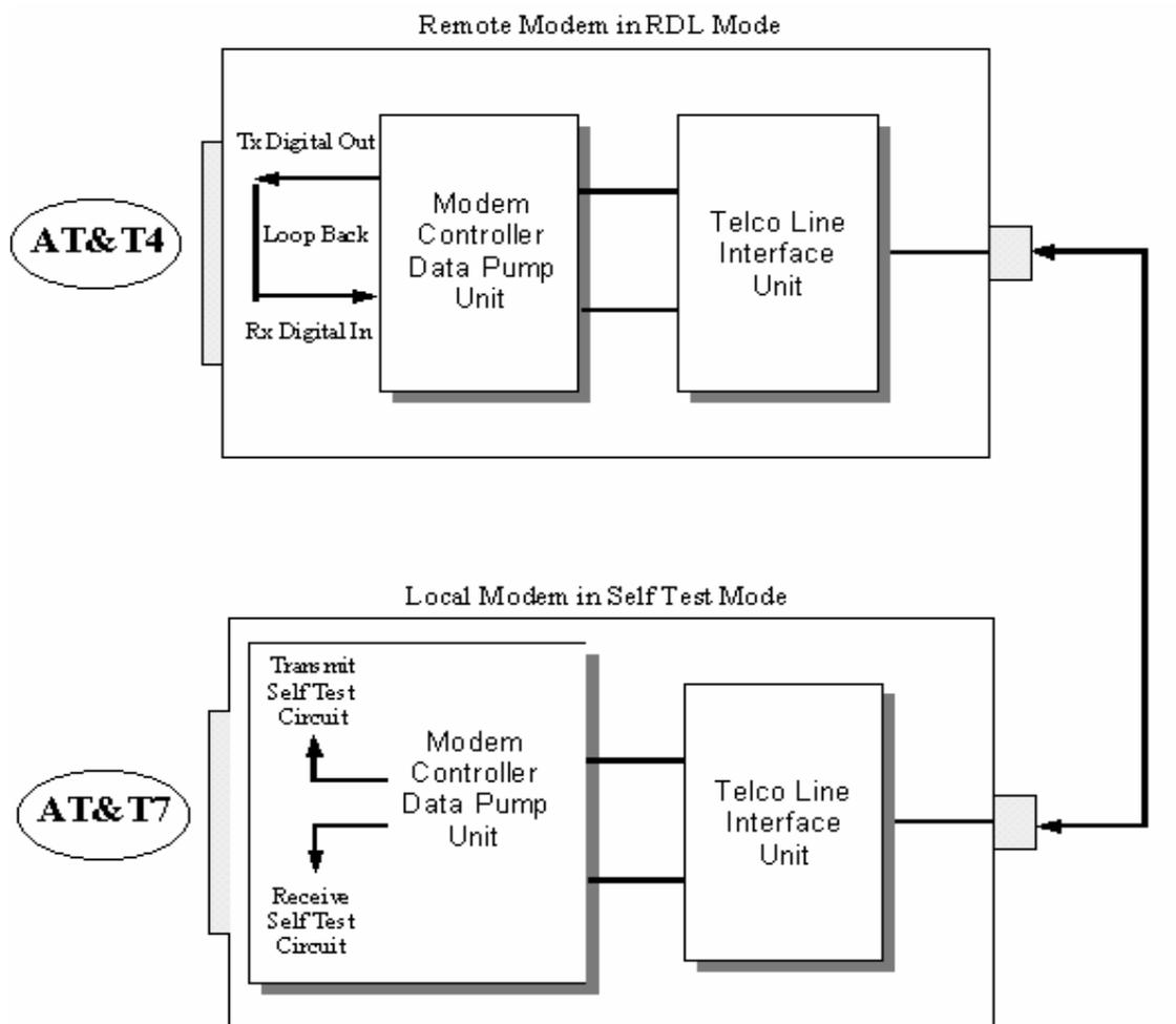
Figure 5 REMOTE DIGITAL LOOPBACK WITH LOCAL SELF TEST
