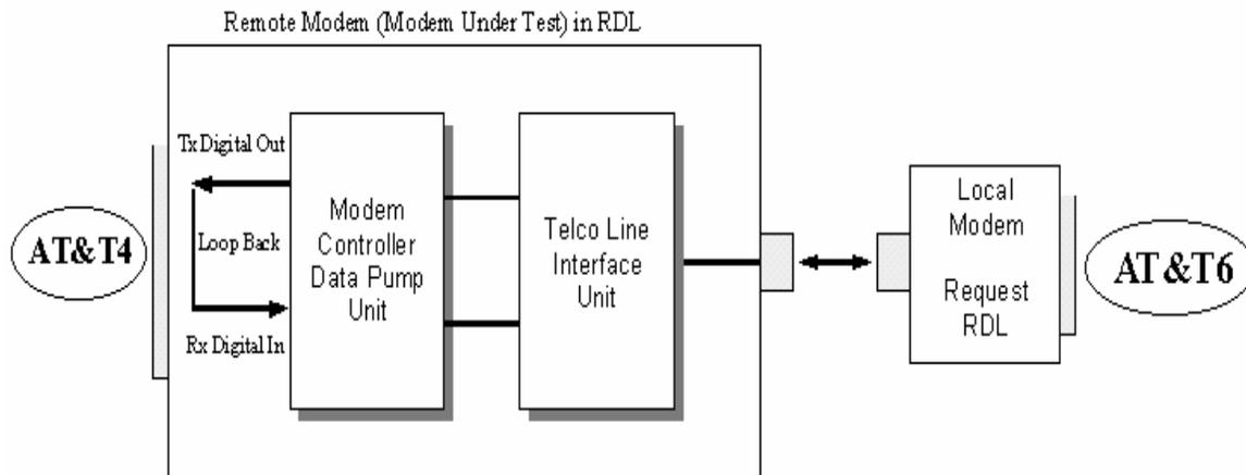
Figure 4 INITIATE REMOTE DIGITAL LOOPBACK
