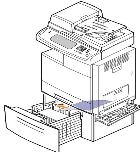
If the jammed paper is not visible, or if the paper is stuck, stop pulling and continue on to step 5.
