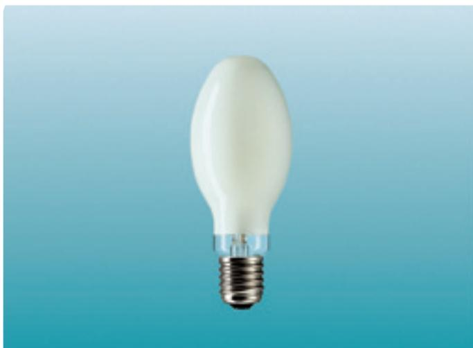
Single ended, high pressure Mercury vapour lamps consisting of a gas-filled soft glass phosphor coated outerbulb. The arc-tube is filled with mercury amalgam. The new HPL 4 Pro lamp achieves maximum light output and peak luminous efficacy at temperatures as low as 15°C, around the lamp. They are therefore particularly suitable for use in outdoor applications especially for those where group replacement costs have a large influence in decision making.
