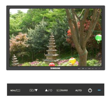
When the 'AUTO' button is pressed, the auto adjustment screen appears as shown in the animated screen on the center.
