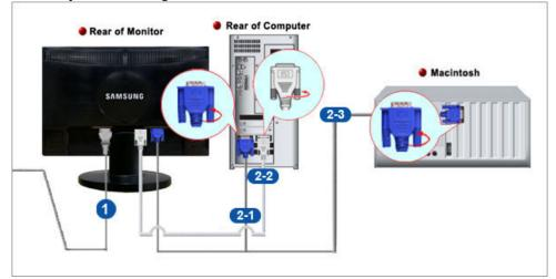
Oconnect the power cord for your monitor to the power port on the back of the monitor.
