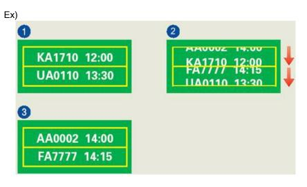
The best way to protect your monitor from Image retention is to set your PC or System to operate a Screen Saver program when you are not using it.
