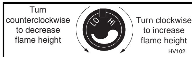
Fig. 34 Flame adjustment knob for Honeywell valve.
