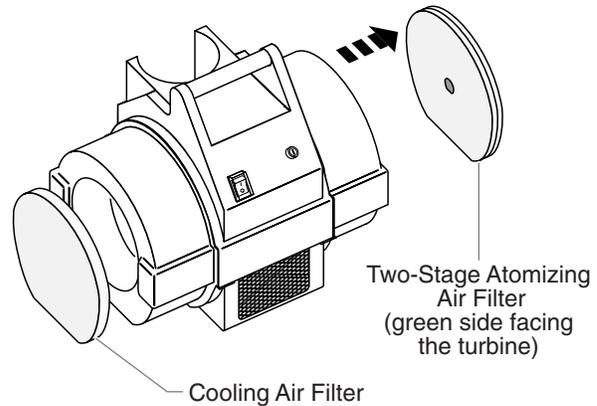
2. Clean the filters. Either tap the filters to knock out the contaminants or use pressurized air to blow out the contaminants. For material that is not blown or knocked loose easily, soak the filters in soapy water or mineral spirits. Allow the filters to dry completely before placing them back in the turbine.
