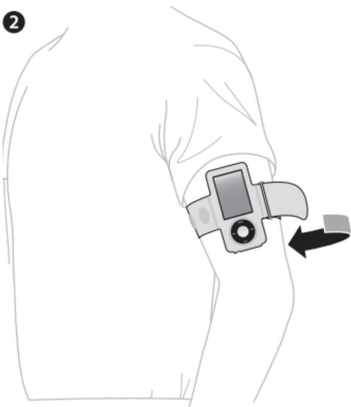
**English:** Slide iPod nano into the armband pocket. Fasten the bottom flap securely. The flap has two settings. Use one if you're using iPod nano alone, and the other if the Nike + iPod receiver is connected.
