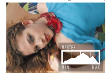
The LCD monitor can be used to display a histogram of any image you take, graphically showing brightness or RGB color distribution among pixels.
