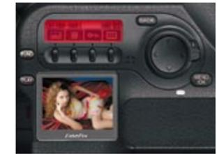
The 1.8-inch low temperature polysilicon TFT-LCD monitor on the back panel of the FinePix S2 Pro delivers crisp, clear images of 130,000 pixels.
