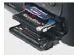
The FinePix S2 Pro is equipped with dual media slots for SmartMedia™ and Microdrive™ cards, letting you concentrate on the shooting without worrying about storage space. You can even insert different types of media in each slot and then select which one you want to use to store each image as you shoot.
