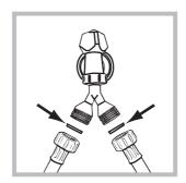
1. Connect the supply pipe to the water mains, fitting the rubber gasket and the filter supplied with the appliance and ensuring that they are fimly tightened to the taps.
