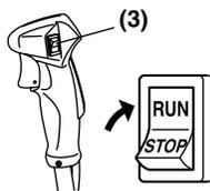
5. **[BCZ3205DL]** Set the stop switch to the "I" position. Set the throttle trigger to the start position (1 → 2 → 3).
