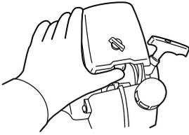
4. Move the choke lever to the closed position.
