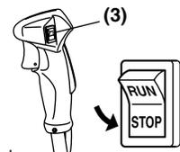
1. Release the throttle trigger and run the engine for half a minute.
