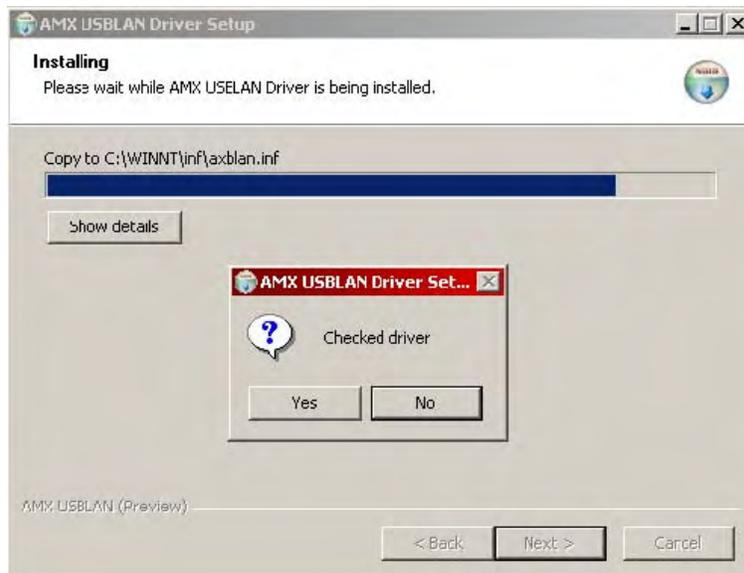
FIG. 6 Do Not Install The "Checked Driver"
