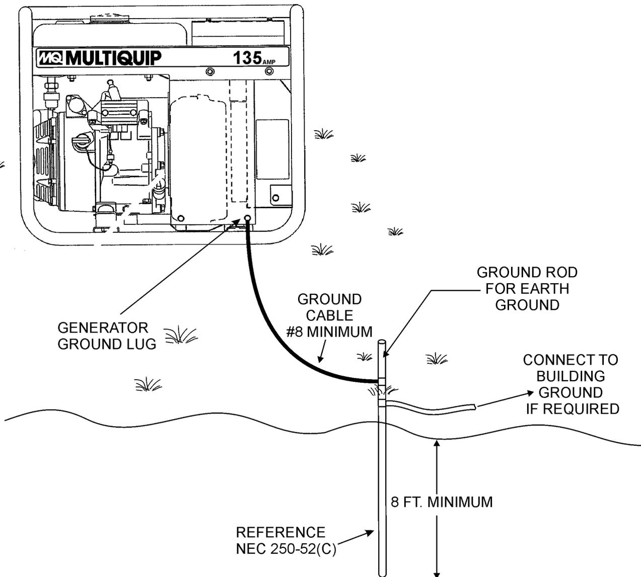
Figure 4. Generator Grounding
