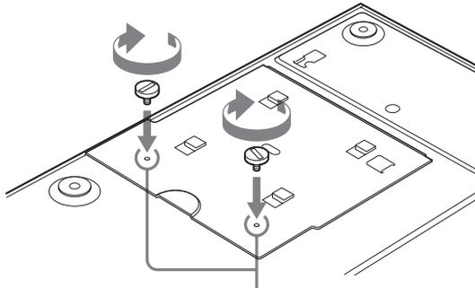
Confirm that the screw holes of the back side of the printer and the back cover plate match before securing them.
