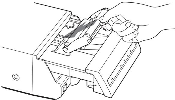
Insert the hole of the handle of the ink ribbon over the protruberance of the printer.
