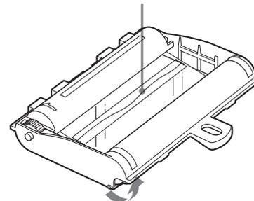
Turn the spools in the direction of the arrow to remove any slack until the transparent tape cannot be seen.
