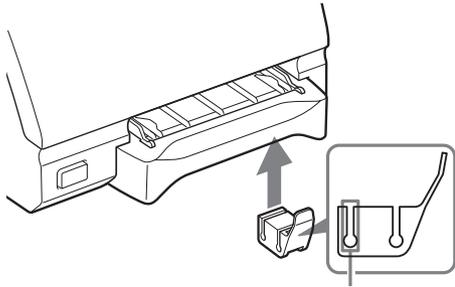
Insert the edge of the paper tray into this groove.
