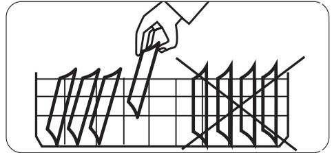
If plates are to be loaded in the upper basket: load them starting from the rear positions; tilting them slightly forwards and avoiding the front positions near the door.
