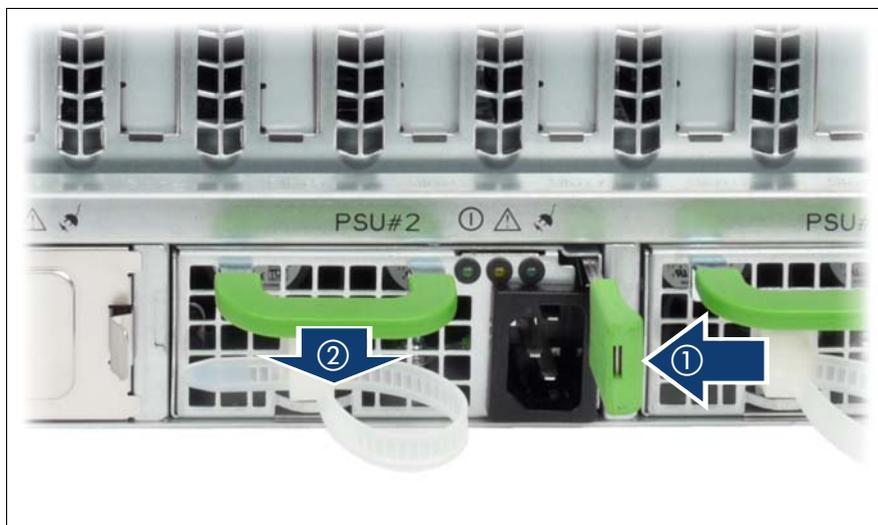
Figure 19: Unlocking and removing the power supply unit
