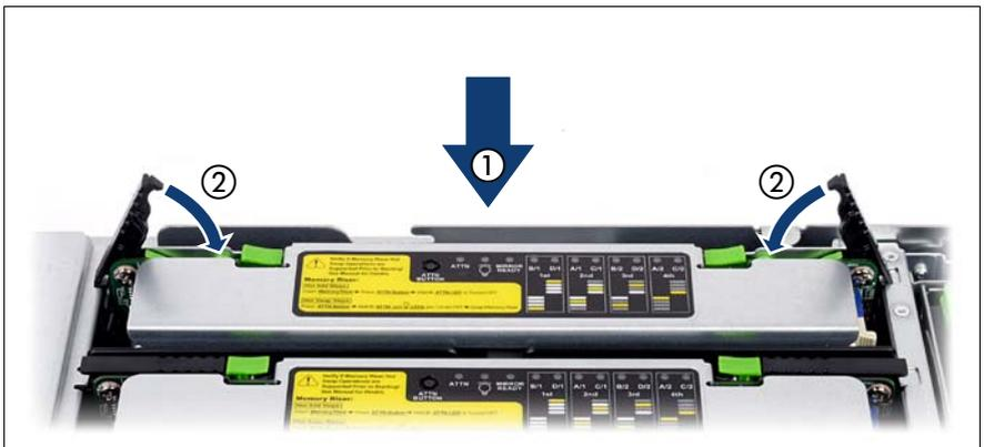
Figure 37: Installing a memory board
