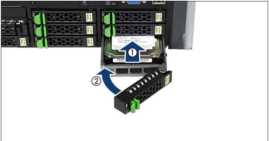
Figure 26: Installing the 2.5-inch HDD module
