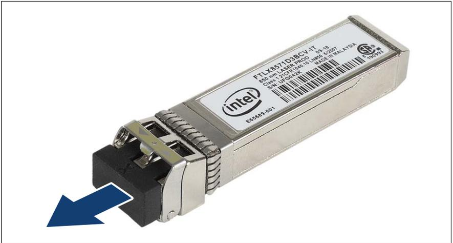
Figure 45: Removing the protective optical port plug
