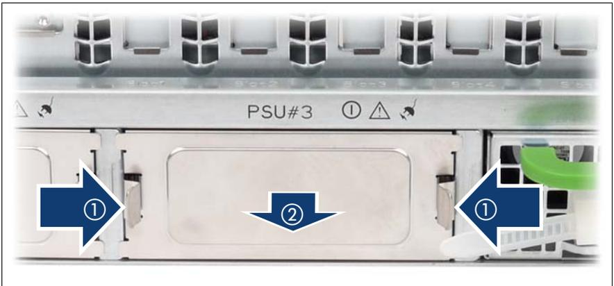
Figure 20: Removing a PSU dummy module
