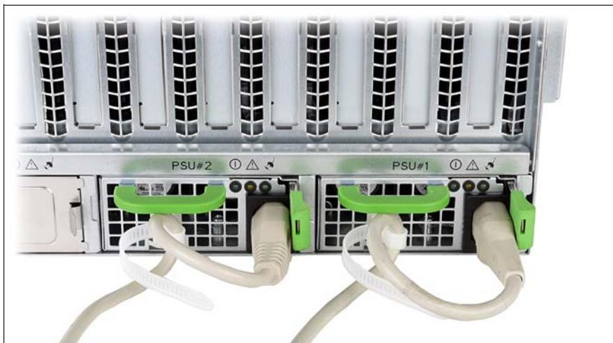
Figure 11: Cable clamps to secure the power cords
