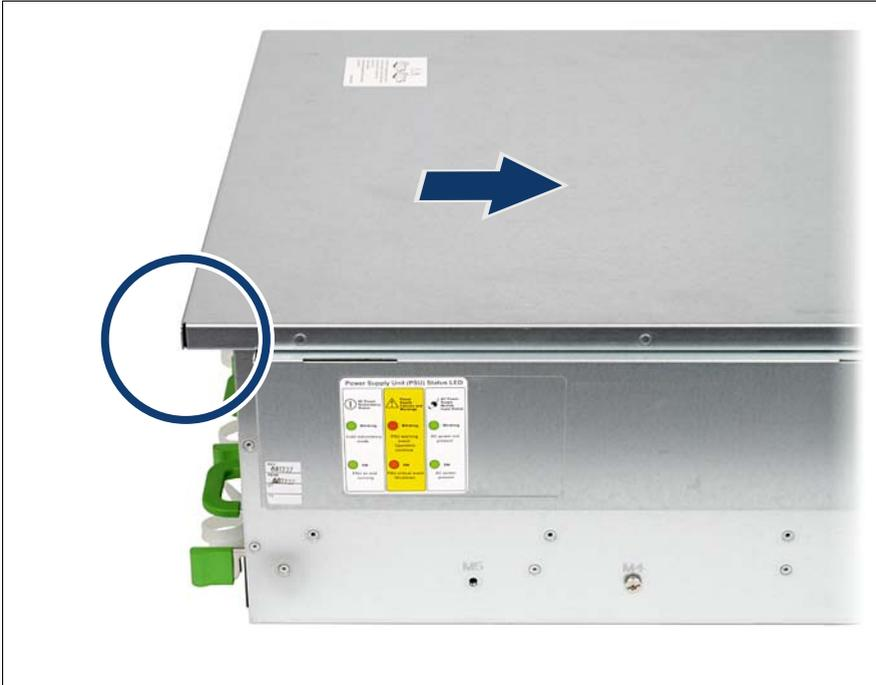
Figure 52: Placing the housing cover
