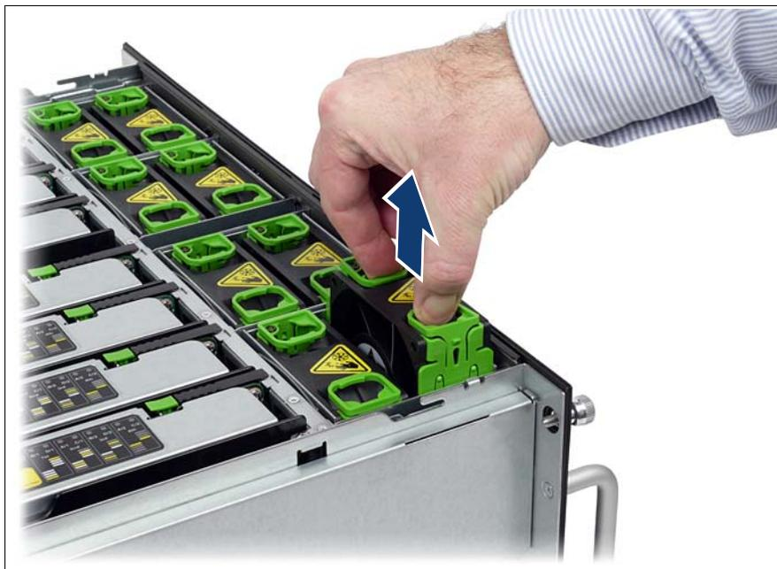
Figure 22: Unlocking a fan module and removing it
