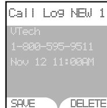
You can also dial a CID record while reviewing. With the desired CID displayed, press **#** or **MENU/SEL**. The possible options to choose from will be either 7, 10, or 11 digits. For example, if the original number in caller ID memory was 800-595-9511, then the display options will be:
