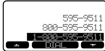
**Dialing Tip:** With a caller ID record displayed, press **#** repeatedly to cycle through the three dialing options. When the correct dialing option is displayed, press **DIAL** or
