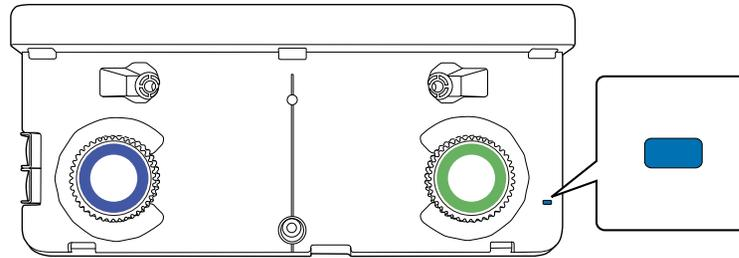
**Warning:** Do not look into the projector's projection window or the Touch Unit's laser diffusion ports (located on the back of the Touch Unit); this could cause injury to eyesight.
