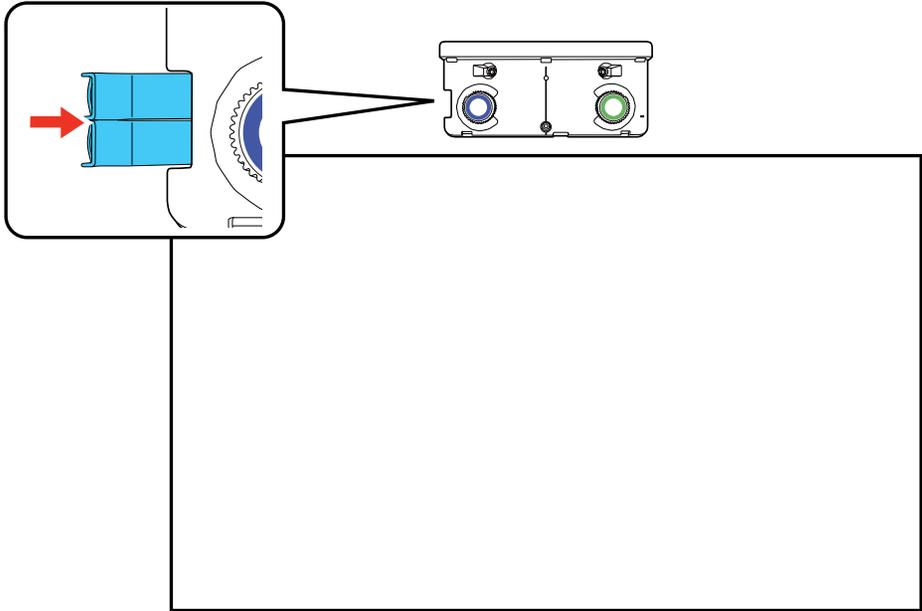
25. Attach the supplied labels to the tabs on either side of the Touch Unit. Match the center of the labels with the tabs on the Touch Unit.
