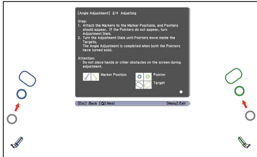
Turning an adjustment dial counterclockwise moves the pointer diagonally down away from the center of the projected image.
