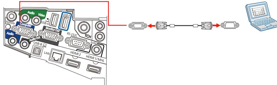
4. Tighten the screws on the VGA connector.
