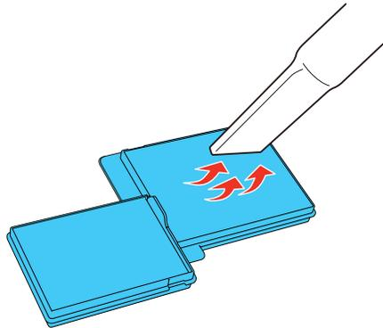
**Note:** If dust is difficult to remove or the air filter is damaged, replace the air filter.
