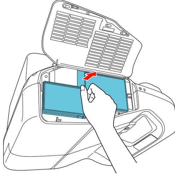
4. Vacuum the front of the air filter (the side with the tabs) to remove any remaining dust.
