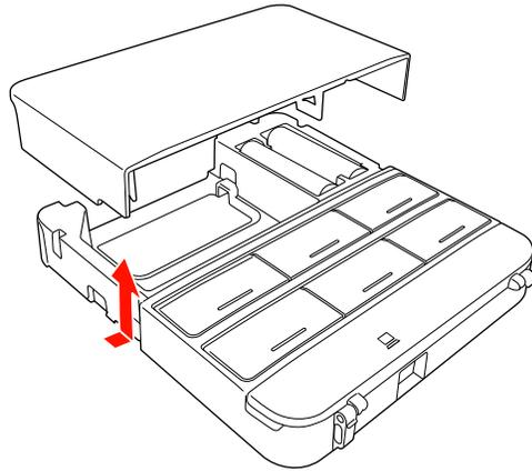
2. Insert the batteries with the + and - ends facing as shown.
