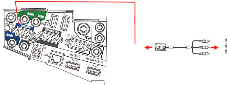
3. Tighten the screws on the VGA connector.
