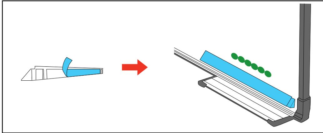
**Note:** Do not remove an infrared deflector once it has been stuck in place. Do not stick tape or place anything on the infrared deflectors. The deflectors will not function properly if anything is placed on them.
