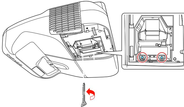
6. Lift up the lamp handle and gently pull the lamp out of the projector.
