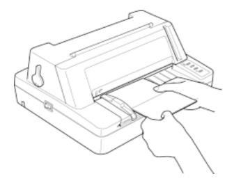
The passbook is fed automatically in to the printer. If the automatic skew correction feature is enable (which it is by default) the passbook will be straightened if it is not inserted correctly.
