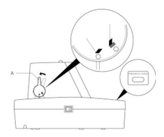
Position the left hand guide in the correct location for the size of paper being used.
