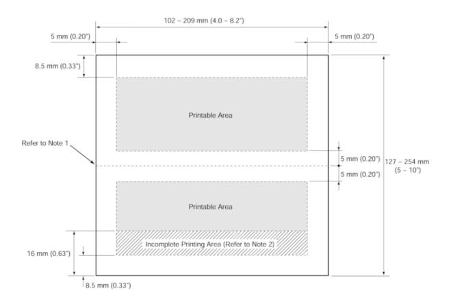
Note 1: Avoid printing in this area to prevent the paper from bending or the ribbon from catching or becoming damaged.
