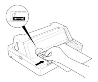
Position the left hand guide in the correct location for the size of paper being used.
