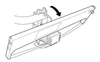
There are two positions for the sensor gap detector. Using the correct position will ensure better paper feeding and also avoid marks on the carbon copy pages of multi-copy media.
