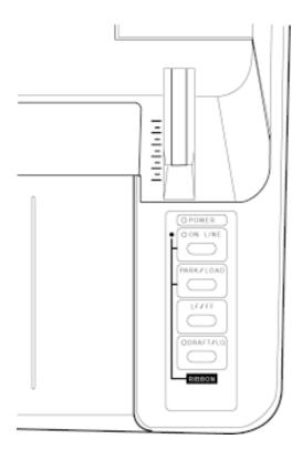
The Printer's control panel consists of 4 keys and 3 indicator LEDs as shown in the diagram to the left.
