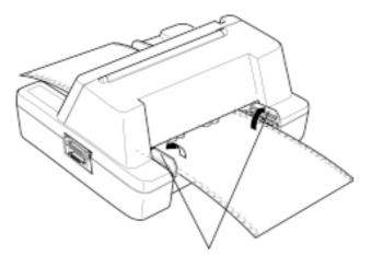
Release the lock lever of left tractor and move the tractor to the left edge of the tractor paper. Fasten the lock lever to lock the tractor in position.
