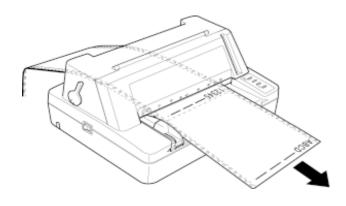
This printer feeds tractor paper from the rear of the printer to the front.
