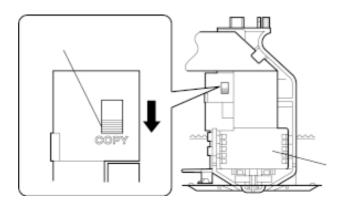
Set the switch in the UPPER position for single sheet fanfold paper, cut sheet and passbooks.
