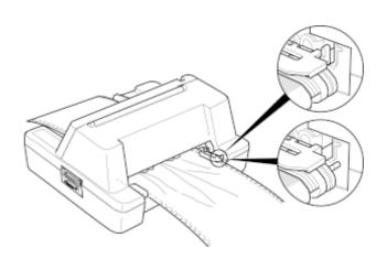
Ensure the tractor paper is in line with the print start position. If the paper is not aligned with the print start position, release the tractor lock levers of the left and right tractors, align the paper, and then fasten the lock lever to lock the tractors.
