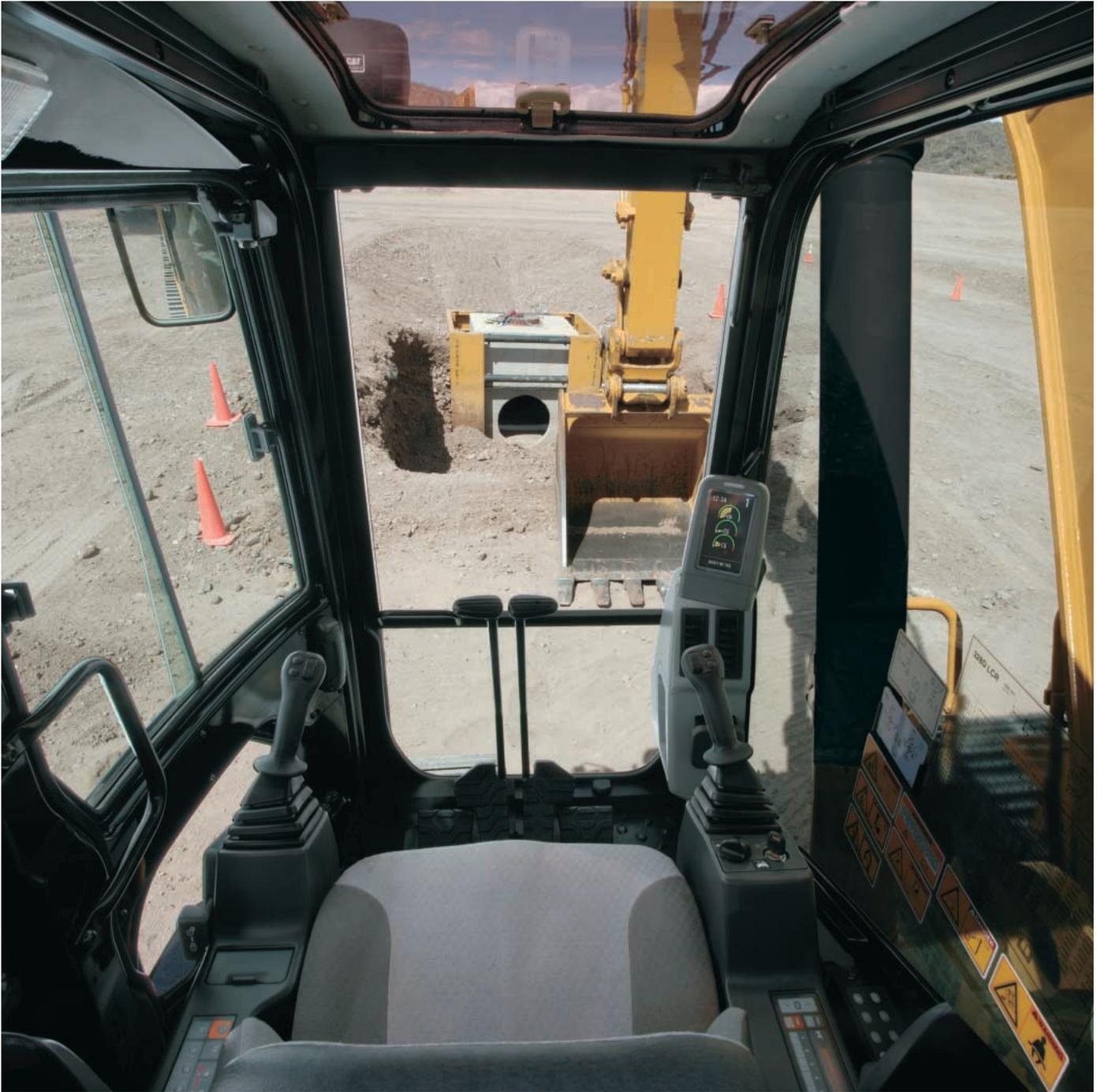
**Operator Station.** The workstation is spacious, quiet and comfortable, assuring high productivity during a long workday. The attachment switches, key switch and throttle dial are conveniently located on the right-hand wall. The monitor is easy to see and maximizes visibility.
