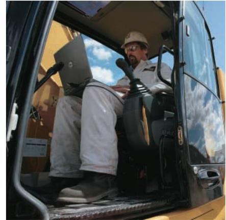
**Diagnostics and Monitoring.** The 328D LCR is equipped with S•O•S<sup>SM</sup> sampling and hydraulic test ports for the hydraulic system, engine oil, and for coolant. A test connection for the Cat Electronic Technician (Cat ET) service tool is located in the cab.
