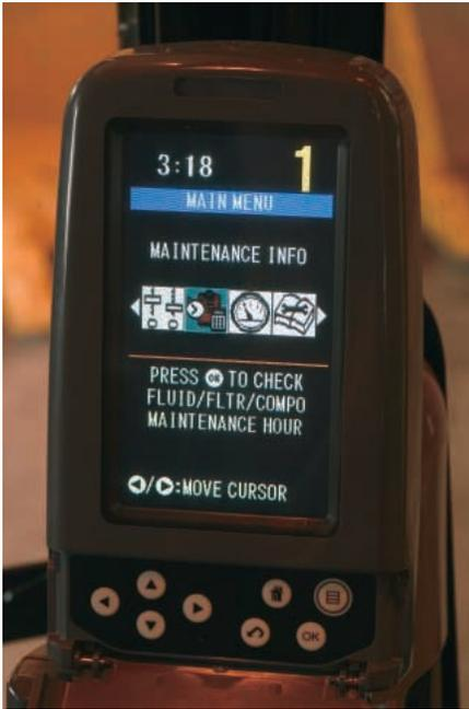
**Monitor.** The monitor is a full color 400x234 pixels Liquid Crystal Display (LCD) graphic display.
