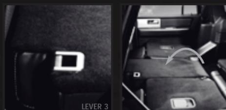
**RETURNING THE 20% MIDDLE SEAT TO THE UPRIGHT POSITION FROM THE FULLY-LOWERED FLOOR POSITION** – To return the seat to the upright position, lift and pull the seat back until the seat latch is fully engaged.
