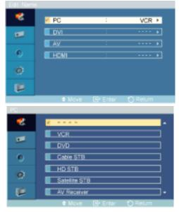
Name the input device connected to the input jacks to make your input source selection easier.
