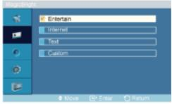
**MagicBright** is a feature providing the optimum viewing environment depending on the contents of the image you are watching. Currently four different modes are available: **Entertain**, **Internet**, **Text** and **Custom**. Each mode has its own pre-configured brightness value. You can easily select one of the four settings by simply pressing the **MagicBright** control button.
