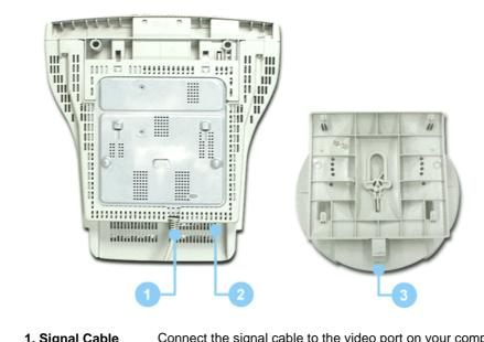
Connect the signal cable to the video port on your computer, video board, video card, or graphics card. 1. Signal Cable
