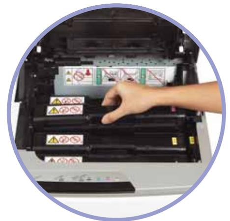
All-in-One Cartridges and a top-loading design make it easy to replace supplies.
