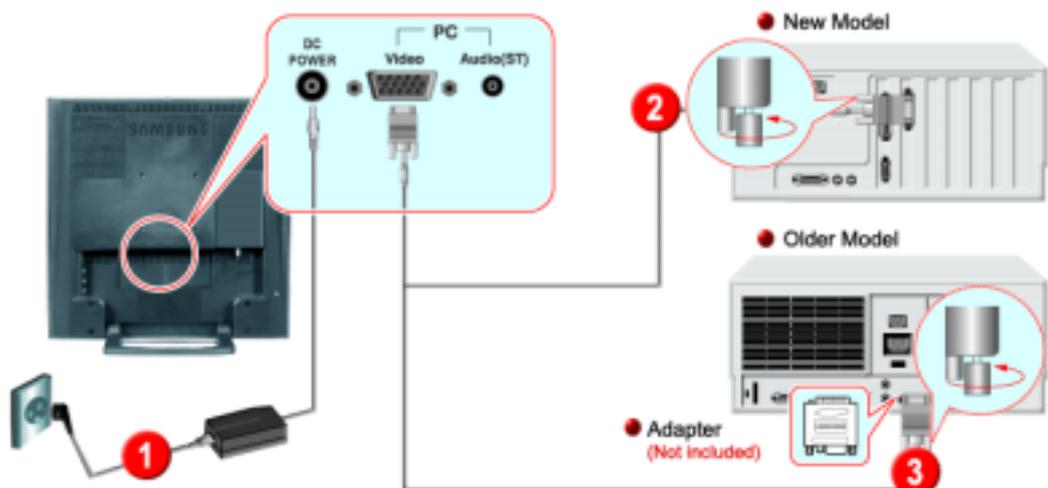
1. Connect the power cord to the DC adapter and then connect the adapter jack to the DC POWER port on the monitor. (Voltage is automatically adjusted by the power adaptor.)
