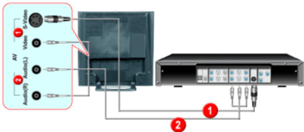
1. Input devices such as DVDs, VCRs or Camcorders are connected to the Video or S-Video terminal of the monitor using the RCA or S-VHS cable.
