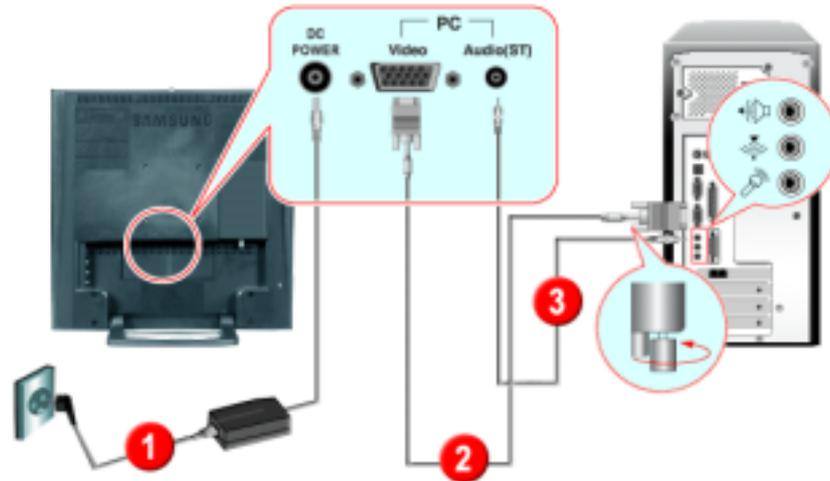
1. Connect the power cord to the DC adapter and connect the adapter jack to the DC POWER port on the back of your monitor.
