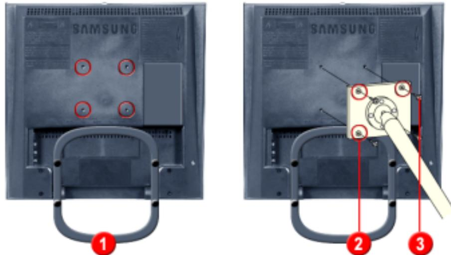
Align **the four bolt holes (1)** on the monitor base with **the holes (2)** on the VESA base and then fasten the base with **the four bolts (3)** supplied.
