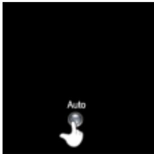
The monitor display becomes more stabilized if adjusted by Auto Adjustment functions when the monitor is installed for the first time. Try Auto Adjustment before attempting Manual Adjustment. Ensure the clock frequency of the monitor matches that of the computer video card before carrying out Auto Adjustment.
