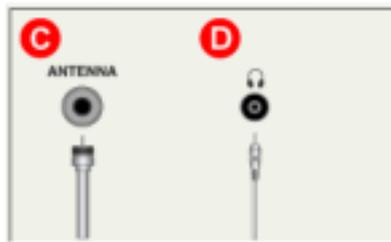
**C. Antenna Connection Terminal (When TV is connected)**
