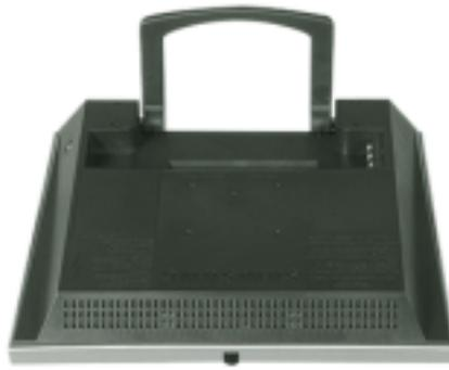
1. Lay the LCD monitor face-down on a flat surface with a cushion beneath it to protect the screen.
