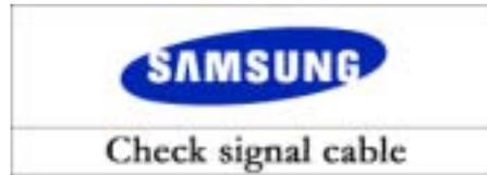
Failure of any of the boxes to appear indicates a problem with your monitor. This box also appears during normal operation if the video cable becomes disconnected or damaged.
