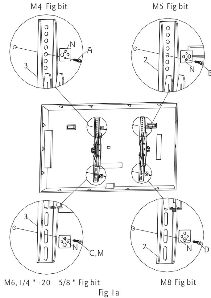
2. Some displays have curved backs with recessed mounting lands (Fig. a). It will require the use of spacer. For this display, install a 9/16" spacer (R) or 1/2" spacer (S) between display and the bracket. As shown in Fig 1b.
