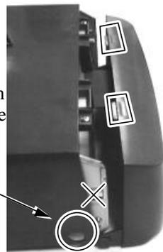
**Note: Never** press the 2 springs on the metal walls as cross marked in the picture. Carelessly pressing on these 2 springs **could cause damages**. The user shall be **responsible** for **such kind of damage**. Even the maintenance technician must always put a piece of clean flat foam of sufficient size in front
