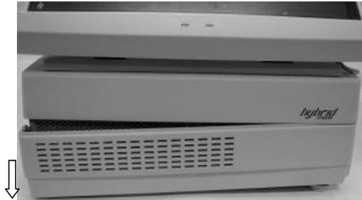
It may be required to push the power switch down to completely remove the front cover.
