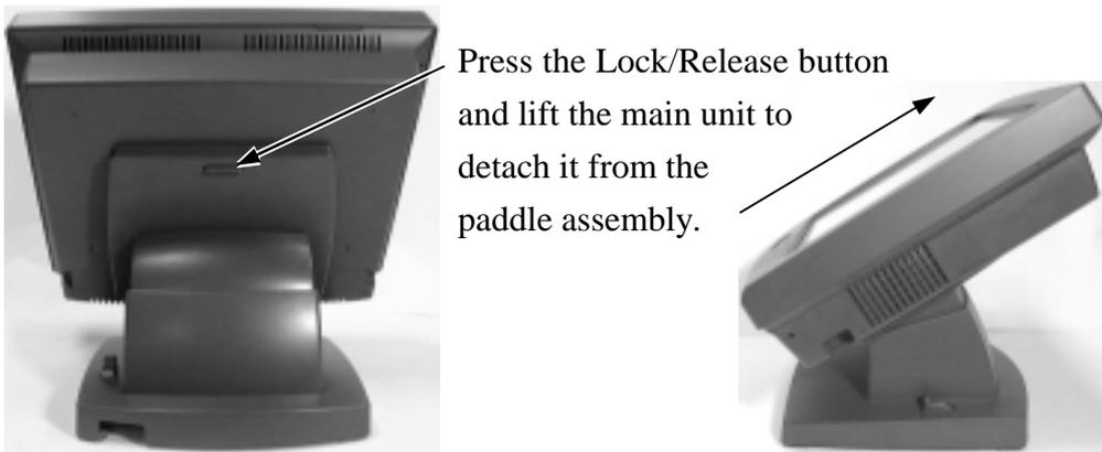
In order to settle the touch terminal properly in a point of sale system, all the cable connections have to be routed through its base, the paddle assembly. Therefore, please press the lock/release button at the rear side to separate the main unit from the paddle assembly.
