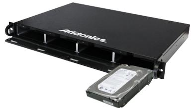
To remove a drive, pull the Eject Lever until the drive disengages from the internal connector then pull the drive out.
