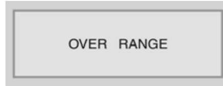
Check that the scanning frequency is in a horizontal range of 24 to 80 kHz and a vertical range of 55 to 75 Hz. Or check that the display resolution is set to 1280 x 1024 or lower.
